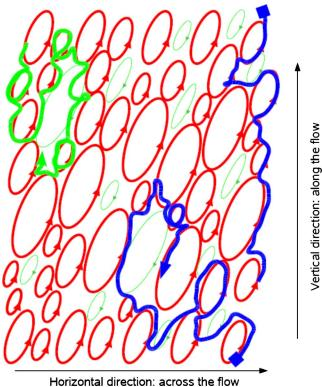
FIG. 12. (Color online) Sketch of motion in the presence of preferential vorticity and eddy tilting. Here, the vertical direction is assumed to be periodic and the periodic continuation of a trajectory is represented by a square. The component of the particle velocity perpendicular to the sheared flow has a larger probability of reversing its direction (over time scales longer than an eddy turnover time) than staying on the same course.
