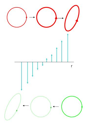
FIG. 11. (Color online) Sketch of the generation of preferential vorticity sign and eddy tilting caused by a sheared flow. Thickness of the line represents the strength of the eddy (i.e., the absolute value of the axial vorticity it contains). The direction of circulation distinguishes between different axial vorticity signs: positive (above) and negative (below).
