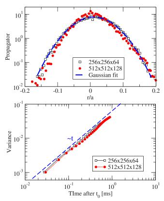
FIG. 10. (Color online) Example of convergence of the transport analysis with respect to grid resolution for the NoF case. Ion guiding-center radial propagators are shown (above) at  $t_0$ +0.12 ms (a Gaussian fit is included for comparison); variance of propagators is also shown as a function of time (below).
