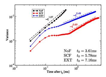
FIG. 8. (Color online) Variance of ion guiding-center radial propagators as a function of the elapsed time after  $t_0$  for cases with NoF, SCF, and EXT driven flow. The values of  $t_0$  used for each case are listed in the lower right corner.
