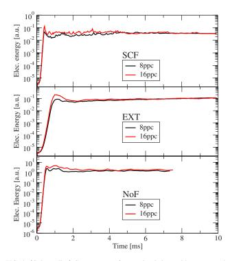
FIG. 4. (Color online) Convergence of UCAN simulations with respect to the number of particles per cell (ppc). All runs have been done with an  $[XYZ] = 256 \times 256 \times 64$  grid. The traces of the total fluctuating electrostatic energy integrated over the whole volume are shown as a function of time. Above: for the SCF case. Middle: for the EXT driven flow case. Below: for the artificially suppressed flow (NoF) case.
