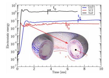
FIG. 3. (Color online) Electrostatic energies for NoF, SCF, and EXT driven flow. Initial  $t_0$  (see text) marked with arrow. Inset: snapshot of temperature fluctuations beyond the linear phase of the self-consistent case just after the zonal flow has already been nonlinearly driven.
