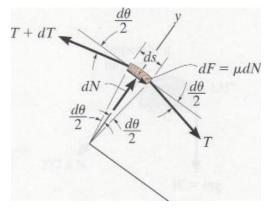
Using this free body digram we will first sum the forces along both the Y and X axis's. Just as a note these are parallel and perpendicular to the normal force and we will be assuming that there is no acceleration (in other words the net forces are zero):
